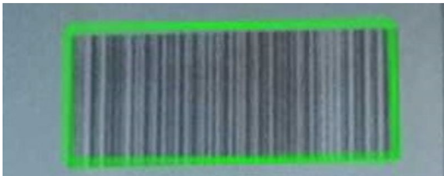
Figure 2 Blurred Code 128 decoded by Viziotix
